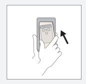
As you move device up into the Guardian case, pull the lower portion of the opening around the bottom portion of the device.
